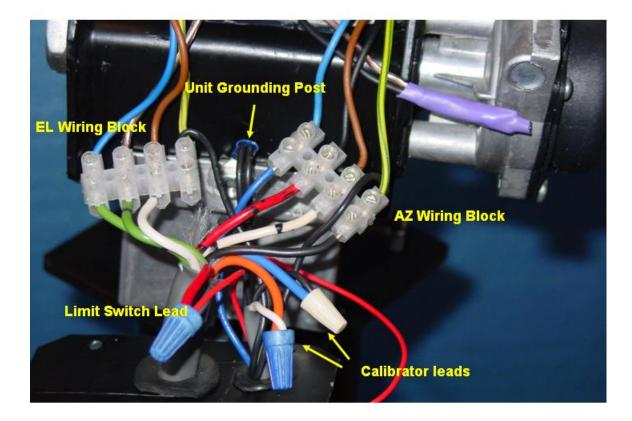
• Carefully stuff the wire assembly back into the AlfaSPID housing and reattach the cover plate.
