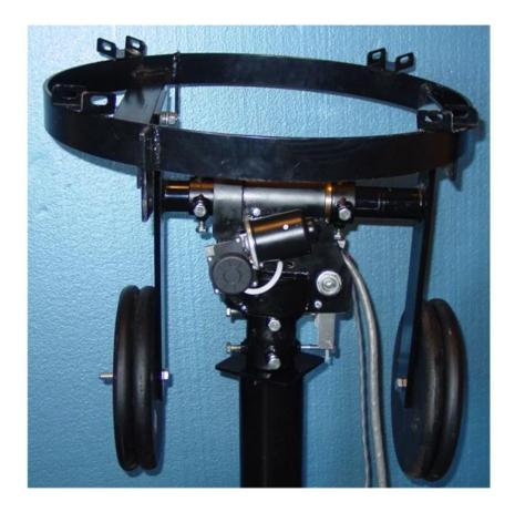
Next lower the dish onto the ring and attach using bolts washers and nuts provided.
