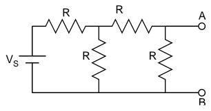
**c.** Determine the equivalent source resistance  $R_{\text{Tot}}$  (sometimes also called the Thevenin resistance) by short-circuiting the output and measuring the current  $I_{\text{sc}}$  through this short-circuit. Sketch (by hand is fine) the  $I(V_{\text{AB}})$  using you the two points obtained in a and b and the above equation.
