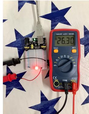
Break circuit, insert Ammeter, read current
