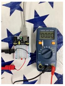
With no or bad Fuse, Ammeter reads zero and LED is off
