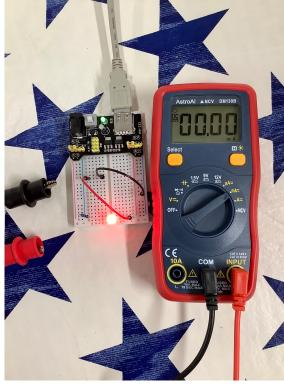
Build circuit with LED and  $100\Omega$  resistor
