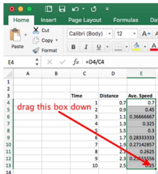
The screenshot shows the same spreadsheet as above, but with the formula =D4/C4 dragged down to fill cells E5 through E13. A red arrow points to the bottom right corner of cell E4 with the text "drag this box down".
