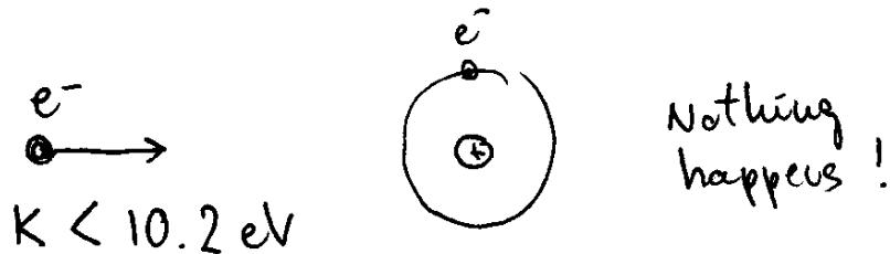
Only if the incident electrons have kinetic energy  $> 10.2 \text{ eV}$ , the excitation process may occur.
