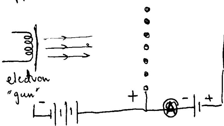
The potential applied between the "electron gun" and the grid accelerates the electrons.
