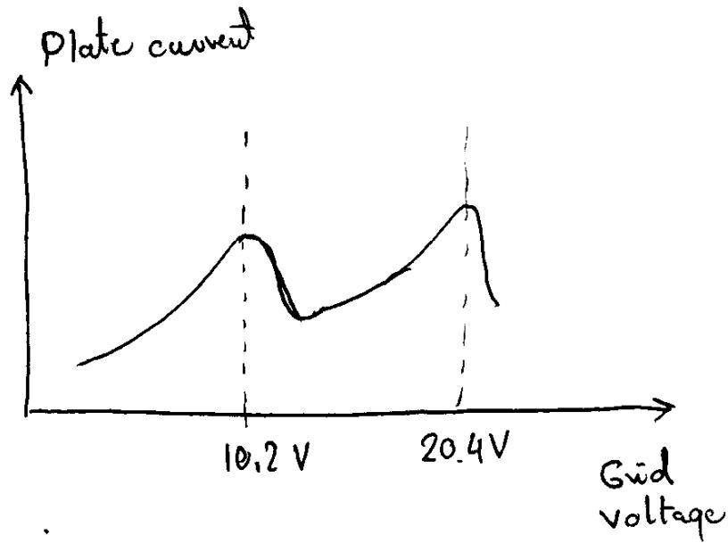
When the grid voltage reaches 10.2 V, there is a sudden "dip" in the plate current.
