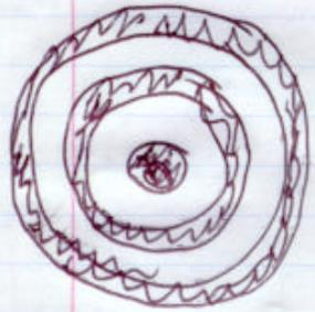
So, when we rotate the apparatus by 90°, then the "ring pattern" goes through a full cycle: black central spot - bright central spot - black central spot again.
