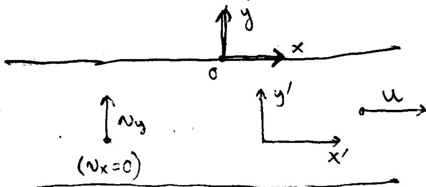
In the frame  $O$  only the velocity component  $v_y$  is non-zero, while  $v_x = 0$ .
