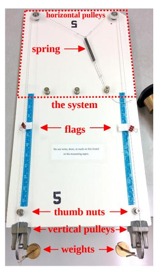
Figure 1: The Partial Derivative Machine. The machine consists of a system which may be manipulated by pulling on two strings. Each string features a flag, which may be used to measure its position, and a weight that can fix the tension in the string. In addition, thumb nuts may be used to fix the position of each string independently.
