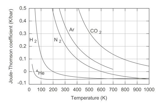
Figure 5.2: Joule-Thomson coefficients  $\mathscr{J}$  for several gases at atmospheric pressure.
