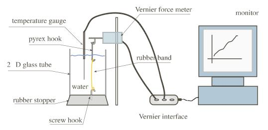
Figure F.1: Experimental arrangement for measurement of  $\tau$  vs. *T*. Add boiling water to the glass tube or fill the tube with acetone and dry ice  $\approx -78$  C. Then allow the system to approach room temperature.
