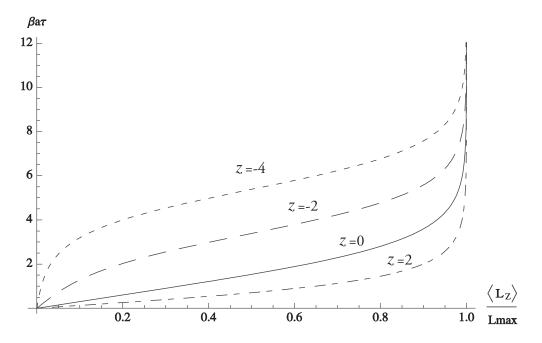
Figure 10.7: Model elastomer stress-strain relationships as described by Eq. 10.78. Curves with  $z = \beta \epsilon < 0$  are typically observed in real rubber-like elastomers.
