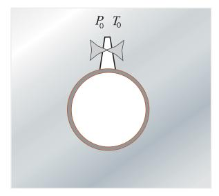
Figure 3.8: Evacuated, insulated vessel in an atmosphere with pressure  $P_0$  and temperature  $T_0$ .
