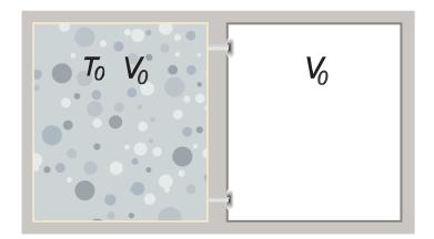
Figure 4.1: Free expansion chamber.
