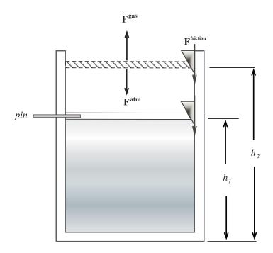
Figure 3.4: Quasi-static irreversible work. A piston slowed by a frictional wedge.
