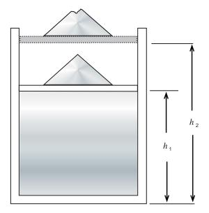
Figure 3.1: Quasi-static reversible work. A piston loaded down with a pile of fine sand.
