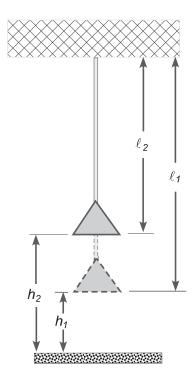
Figure 3.6: A loaded, constrained rubber band when suddenly released rapidly contracts.
