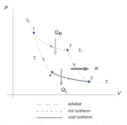
Figure 4.4: An ideal Carnot engine cycle drawn in the P-V plane.
