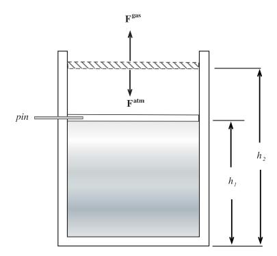
Figure 3.3: Irreversible work. A gas-filled piston initially pinned at height  $h_1$ .
