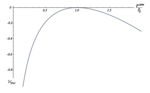
Figure 3.5: Work  $\mathcal{W}_{frict}$  done by the frictional wedge .
