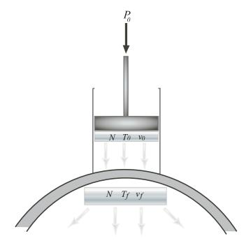
Figure 3.9: Evacuated vessel filling under pressure  $P_0$ .
