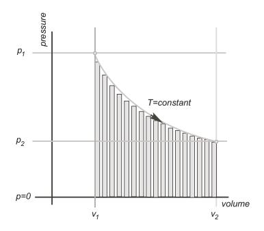
Figure 3.2: p - V diagram for an isothermal quasi-static process.
