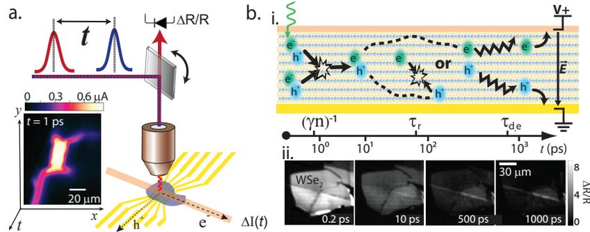
**Fig. 1. Experimental setup and timeline for charge extraction.** (a) In the WSe<sub>2</sub> device shown, we measure the exciton dissociation dynamics with U-PC,  $\Delta I(t, V)$  and TA,  $\Delta R(t, V)$ . (inset)  $t = 1$  ps scanning U-PC spatial map. (b) i. Cutaway of device geometry, with transparent top gate held at voltage  $V$ . It depicts a timeline of photocurrent generation events. ii. Scanning TA microscopy maps of few-layer WSe<sub>2</sub> show electron recombination.
