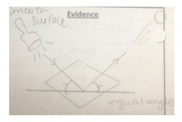
Light from the source bounces off of the smooth surface (such as a mirror) in such a way that the angles created by the light are equal. These angles, called the angle of incidence and the angle of reflection, are equal.
