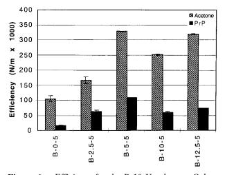
**Figure 6.** Efficiency for the B-10-X columns. Calculations are based on peak width at half height. Experimental conditions are as in Table II.
