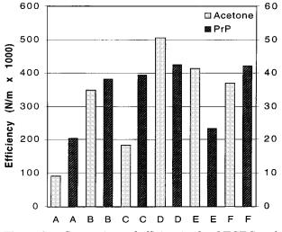
**Figure 8.** Comparison of efficiencies for OTCEC and OTLC. Left axis: efficiencies for acetone, an unretained test probe. Right axis: efficiencies for PrP, a retained test probe. Experimental conditions are as displayed in Figure 7.
