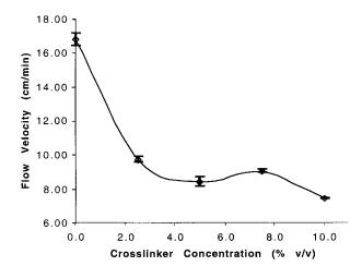
**Figure 2.** Flow velocities for the B-10-X columns. Data points represent the mean of five measurements, error bars represent  $\pm 1$  standard deviation. Capillary:  $L_{TOT} = 37$  cm,  $L_{DET} = 30$  cm. Potential applied: 30 kV constant, positive polarity. Measurements were performed using a Beckman CE system. Other experimental conditions are indicated in the text.
