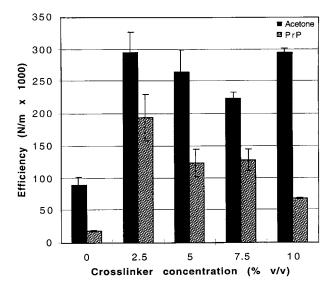
**Figure 5.** Efficiency for the B-10-X columns. Calculations are based on peak width at half height. Experimental conditions are as in Figure 2.
