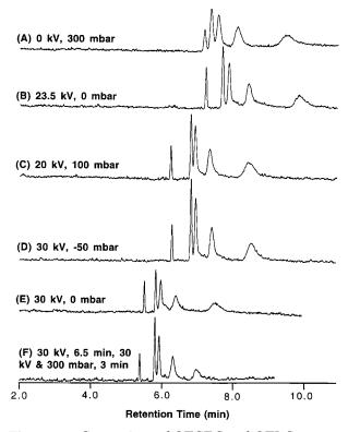
**Figure 7.** Comparison of OTCEC and OTLC separations. Capillary: B-15-15,  $L_{TOTAL} = 60$  cm,  $L_{DEC} = 45$  cm. Other conditions are as in Figure 1.
