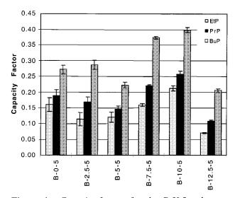
**Figure 4.** Capacity factors for the B-X-5 columns. Data points represent the mean of five measurements, error bars represent  $\pm 1$  standard deviation. Experimental conditions are as indicated in Table II.
