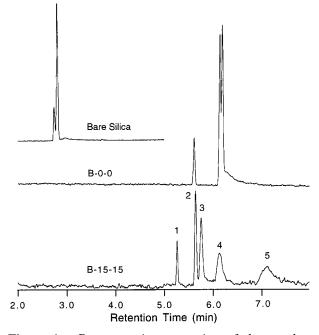
**Figure 1.** Representative separation of the paraben mixture. Capillary:  $L_{TOTAL} = 60$  cm,  $L_{DET} = 45$  cm. Applied potential: 30 kV, positive polarity. Peaks: (1) acetone; (2) MeP; (3) EtP; (4) PrP; (5) BuP. Data were collected on an ATI CE system. Other conditions are listed in the text. The signal (Y) axis is compressed for the bare silica and B-0-0 capillaries.
