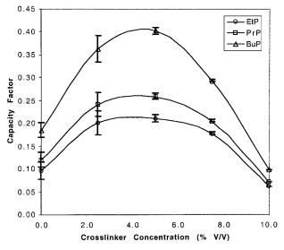
**Figure 3.** Capacity factors for the B-10-X columns using parabens as test solutes. Data points represent the mean of five measurements, error bars represent  $\pm 1$  standard deviation. Other experimental conditions are as indicated in Figure 1.
