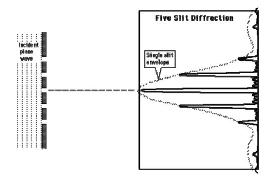
Comparison of single and multiple slit diffraction Fig. LN3A-2. Single- and Multiple Slit Diffraction. taken from <u>http://hyperphysics.phy-astr.gsu.edu/hbase/phyopt/mulslid.html#c3</u>
