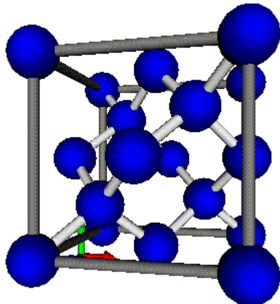
There are 2 C atoms in the diamond lattice at (0,0,0) and (1/4,1/4,1/4). There is more than one way to calculate the C-C distance. One that is very easy is to the distance formula in 3D:
