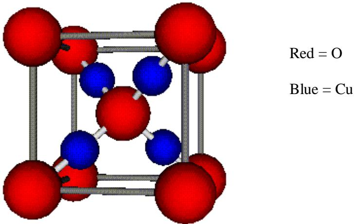
Notice that there are O atoms at the cell vertices that are symmetrically equivalent to (0,0,0).
