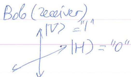
Bob has a polarizer to separate polarization onto two detectors  $\Rightarrow$  when he gets a photon in a vertically polarized detector  $\Rightarrow$  "1"
